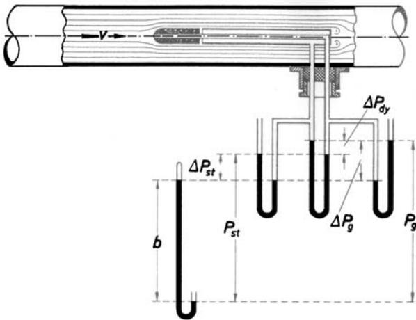
The **STATIC PRESSURE  $P_{st}$** : is the internal pressure of a flowing gas or that pressure which a gas flowing parallel to the wall of the conduit is exerting on the same. Through a suitable boring in the wall of the pipe or the duct, or through the ring-shaped slit of a Pitot tube, it can be measured as absolute pressure  $P_{st}$  or as pressure difference  $\Delta P_{st}$  compared to the free atmosphere.
