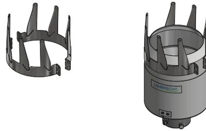
Bend the chain stays while the ring is mounted on the rain[e]
