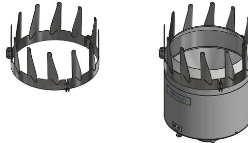
Bend the chain stays while the ring is mounted on the rain[e]
