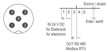
Cable-side socket (female) M12 4-pin, shielded
